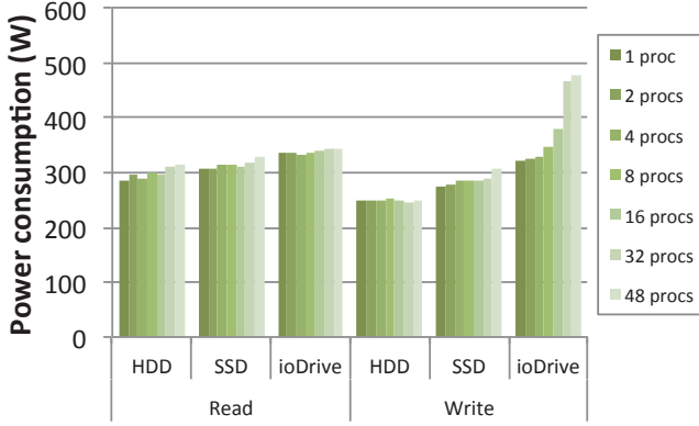
Figure 4: Power consumption with different number of processes and devices
